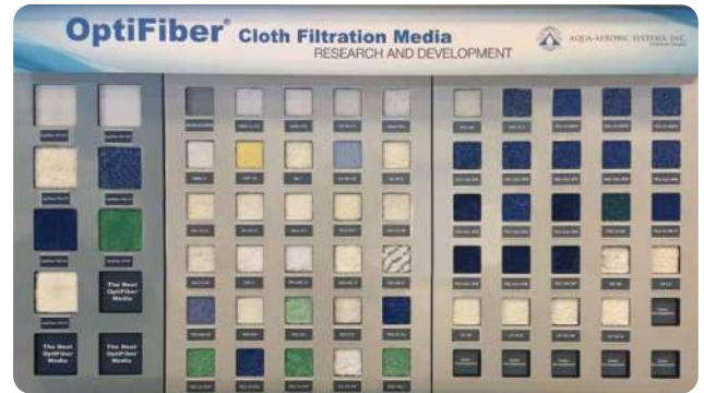
A cloth media display showcases samples of tested media with the far left panel featuring OptiFiber® media.
