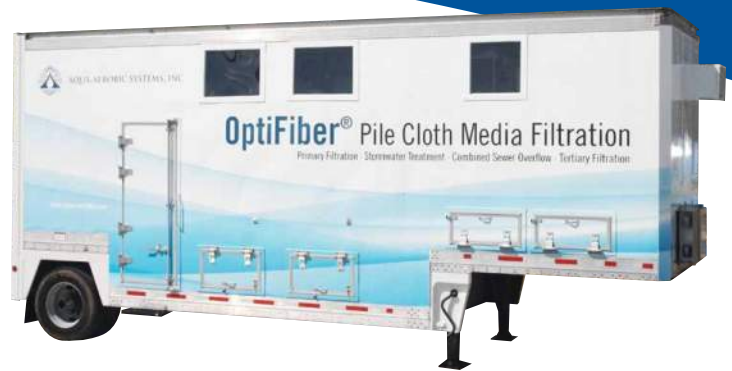
Mobile Primary Filtration Pilot System
