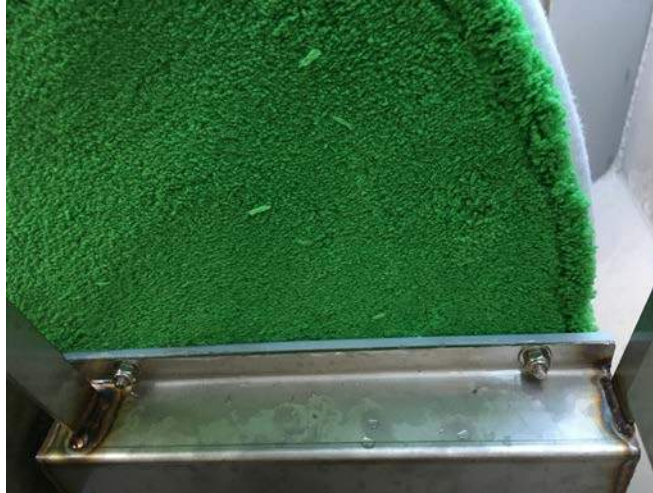
Figure 2: OptiFiber PF-14 ® Cloth Filtration Media
