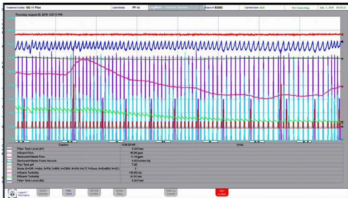
Figure 1: Screen shot of online SCADA data collection for primary treatment application.
