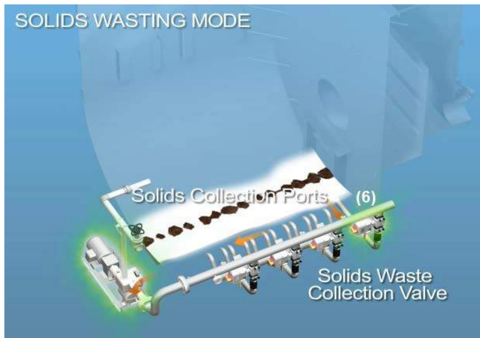
Settled Solids Removal
