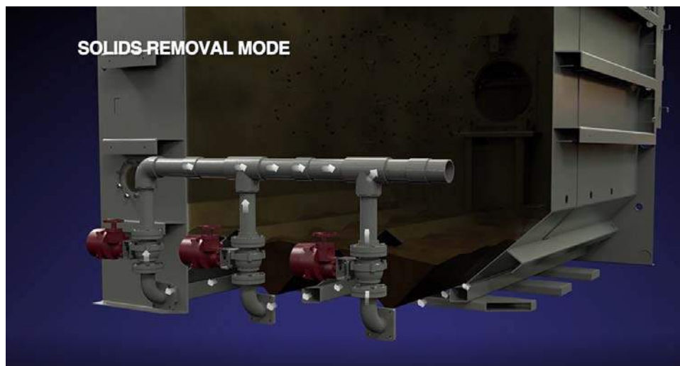
Figure 8: Solids Removal Mode – Pumping of solids out of System
