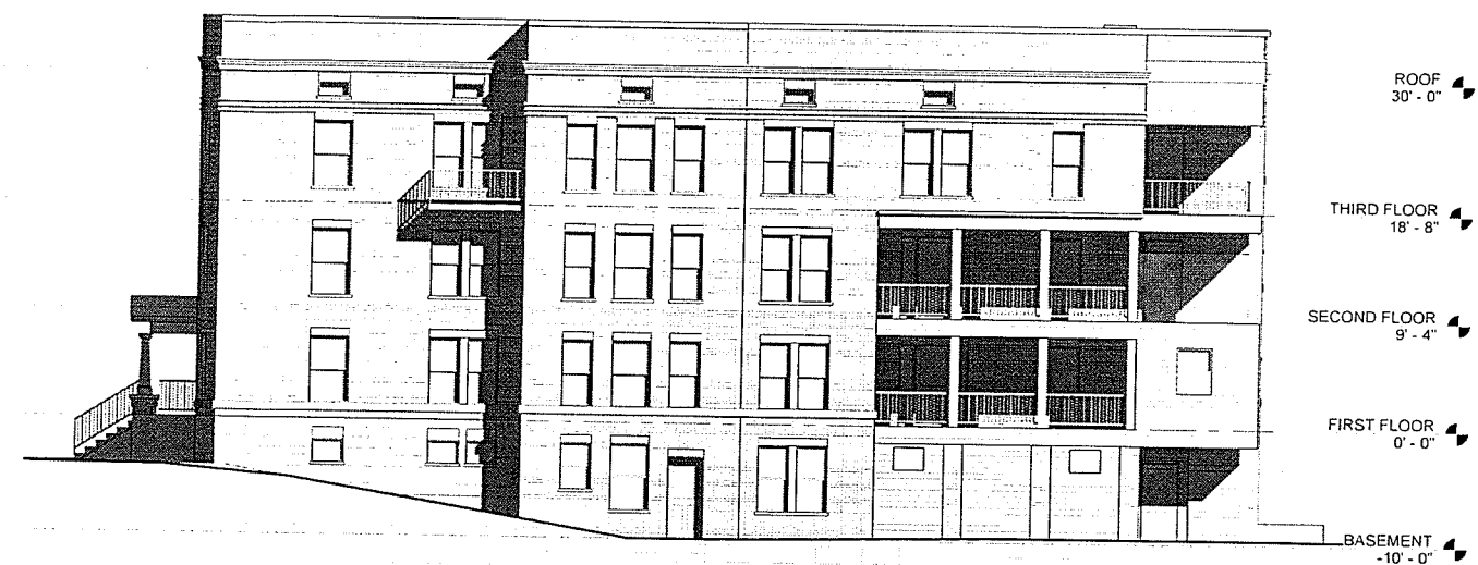
2 EXISTING WEST ELEVATION 1/8" = 1'-0"
