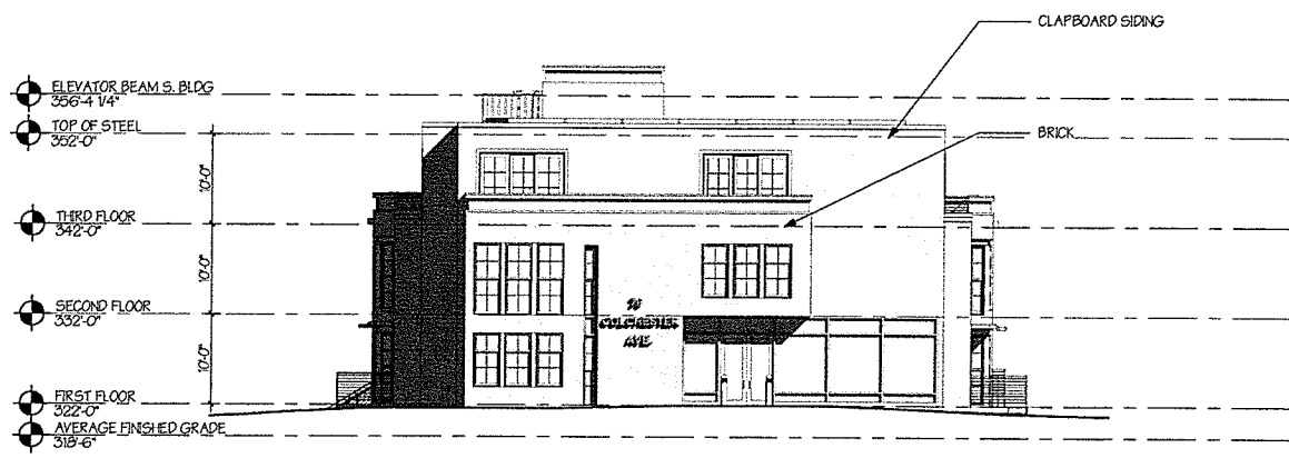
3 SOUTH ELEVATION BLDG 2 3/32" = 1'-0" Referenced From: A102
