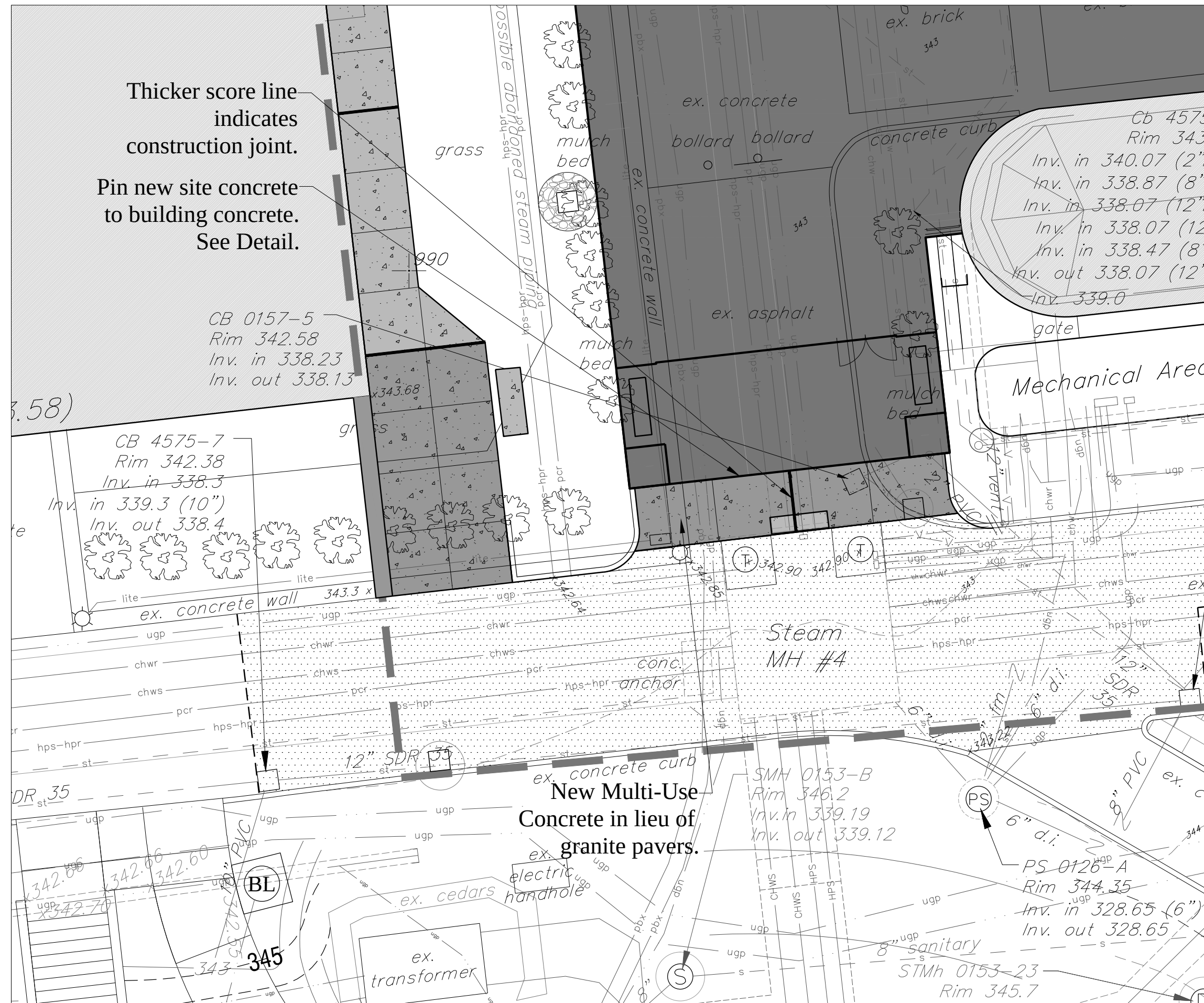
Alternate C-2 - South Entrance Concrete Pavement
