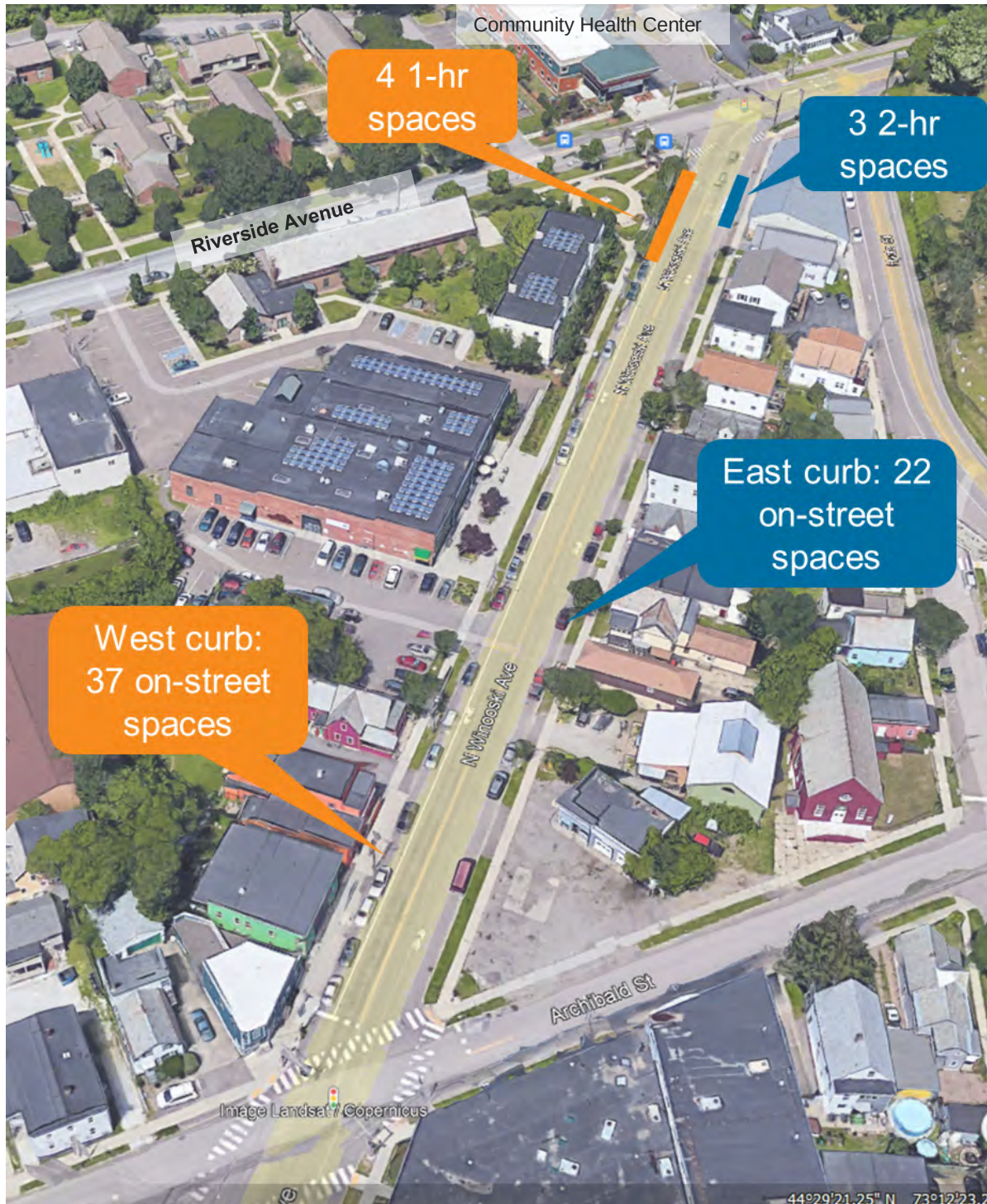
FIGURE 17: EXISTING PARKING CONDITIONS: RIVERSIDE TO ARCHIBALD
