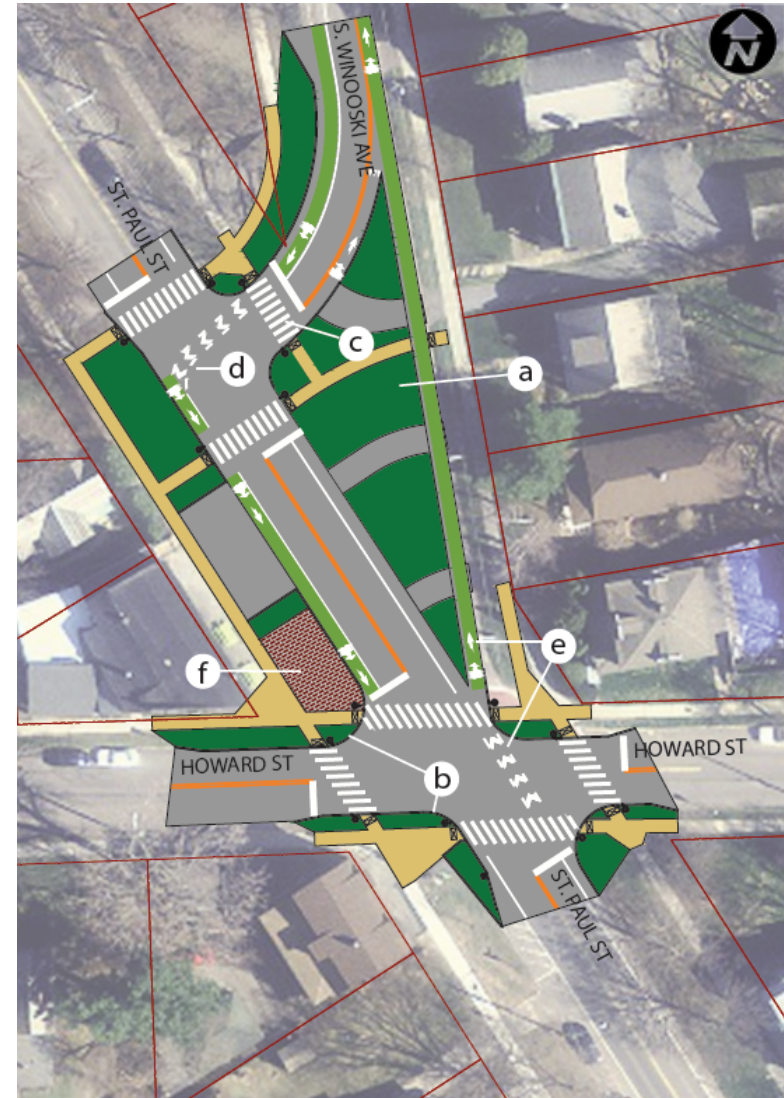
FIGURE 11-6: NEW SIGNAL SYSTEM, REALIGNED ROADWAY
