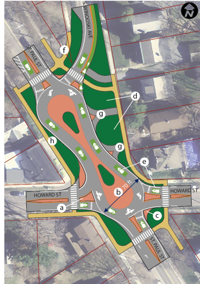
FIGURE 11-8: DUAL ROUNDABOUT, REALIGNED ROADWAY
