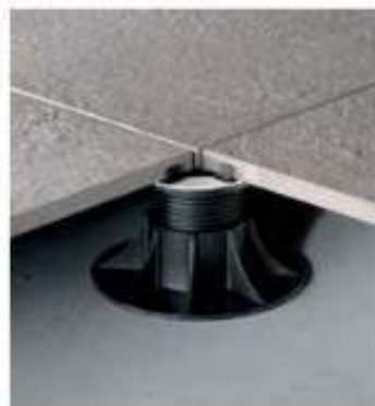
SELF-LEVELLING HEIGHT: from 37.5mm to 100mm; compensates for inclinations up to 5%
