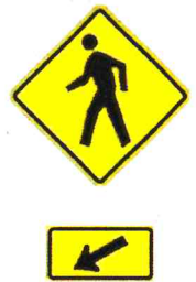
Figure 32: Recommended Pedestrian Warning Signs (MUTCD W11-2 and W16-7P)
