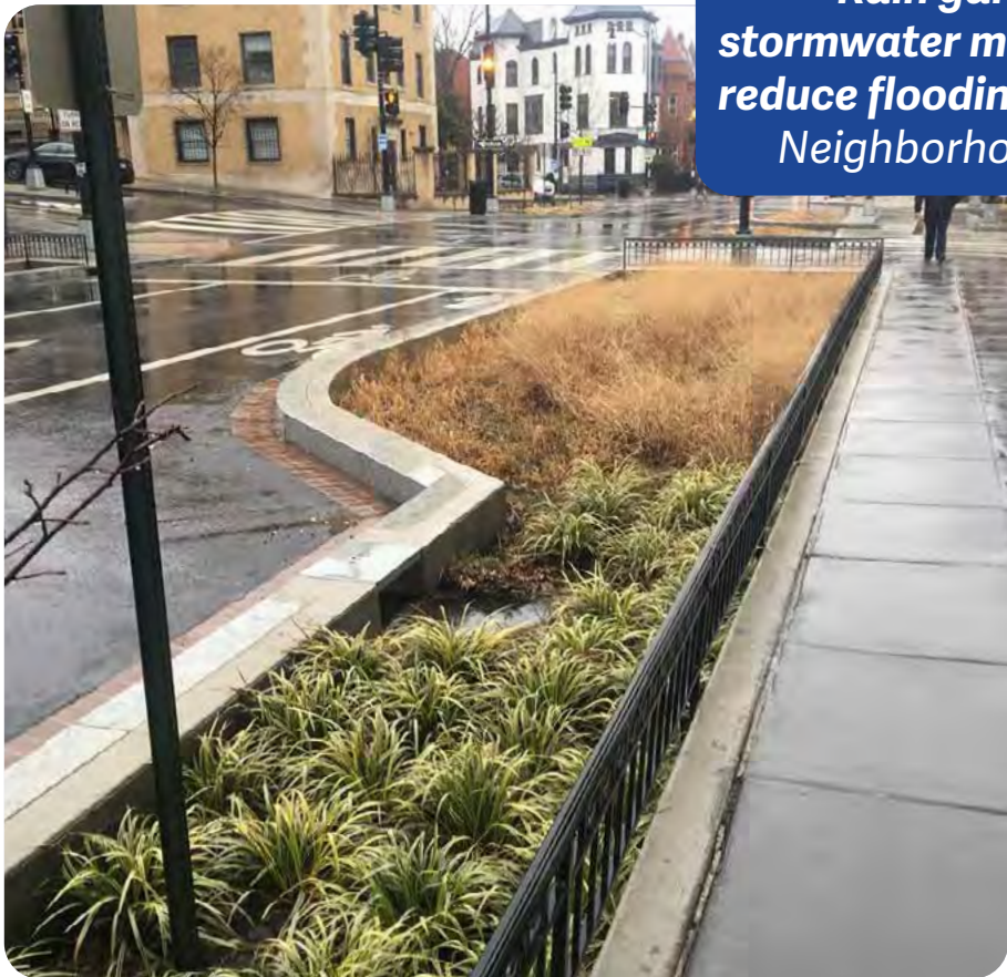
Stormwater retention focused at lowpoints near edges and nodes
