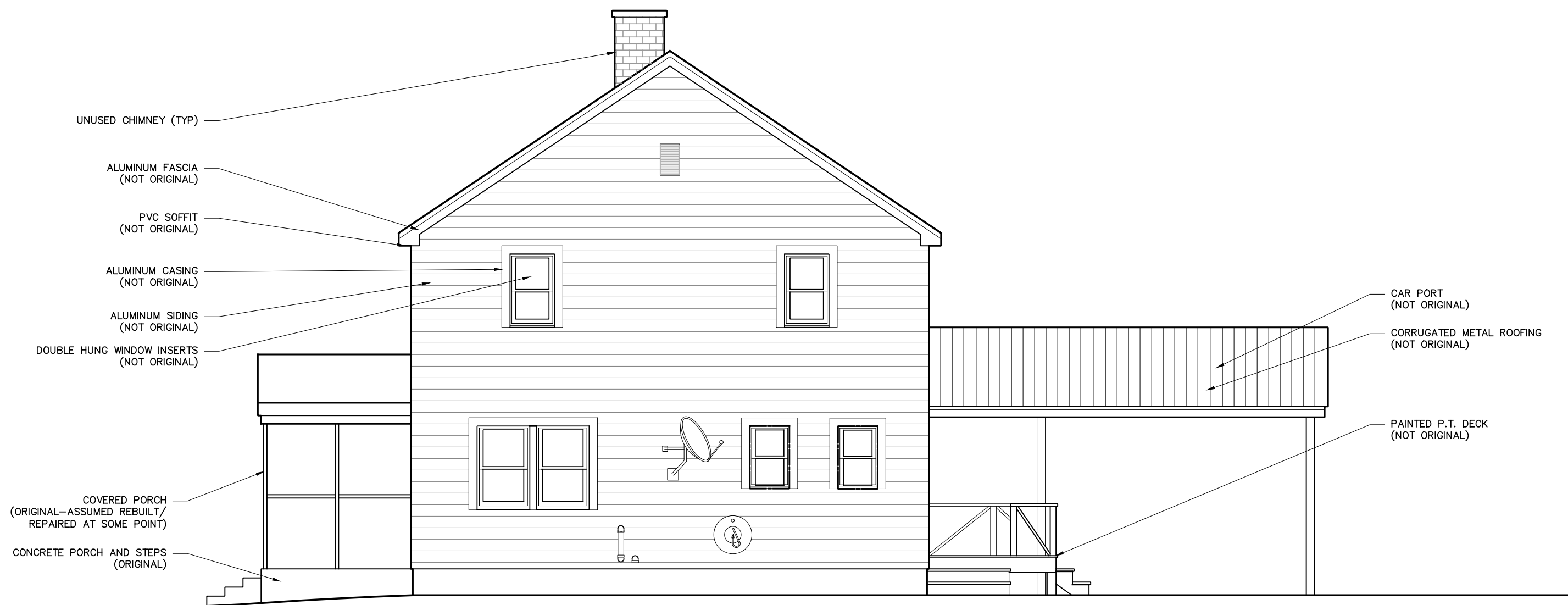
2 EXISTING WEST ELEVATION - SIDE
