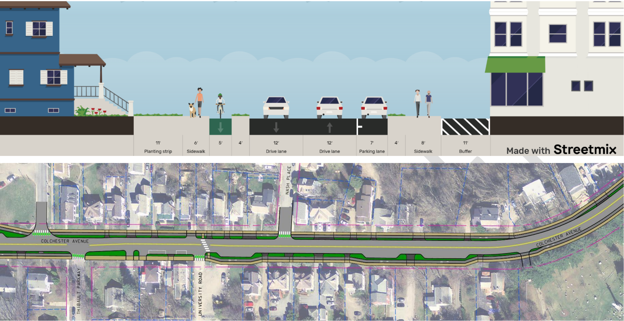
Figure 15: Colchester Ave Corridor Concept 3A (East): Raised, Separated Bike Lanes with Enhancements and Mixing Zone
