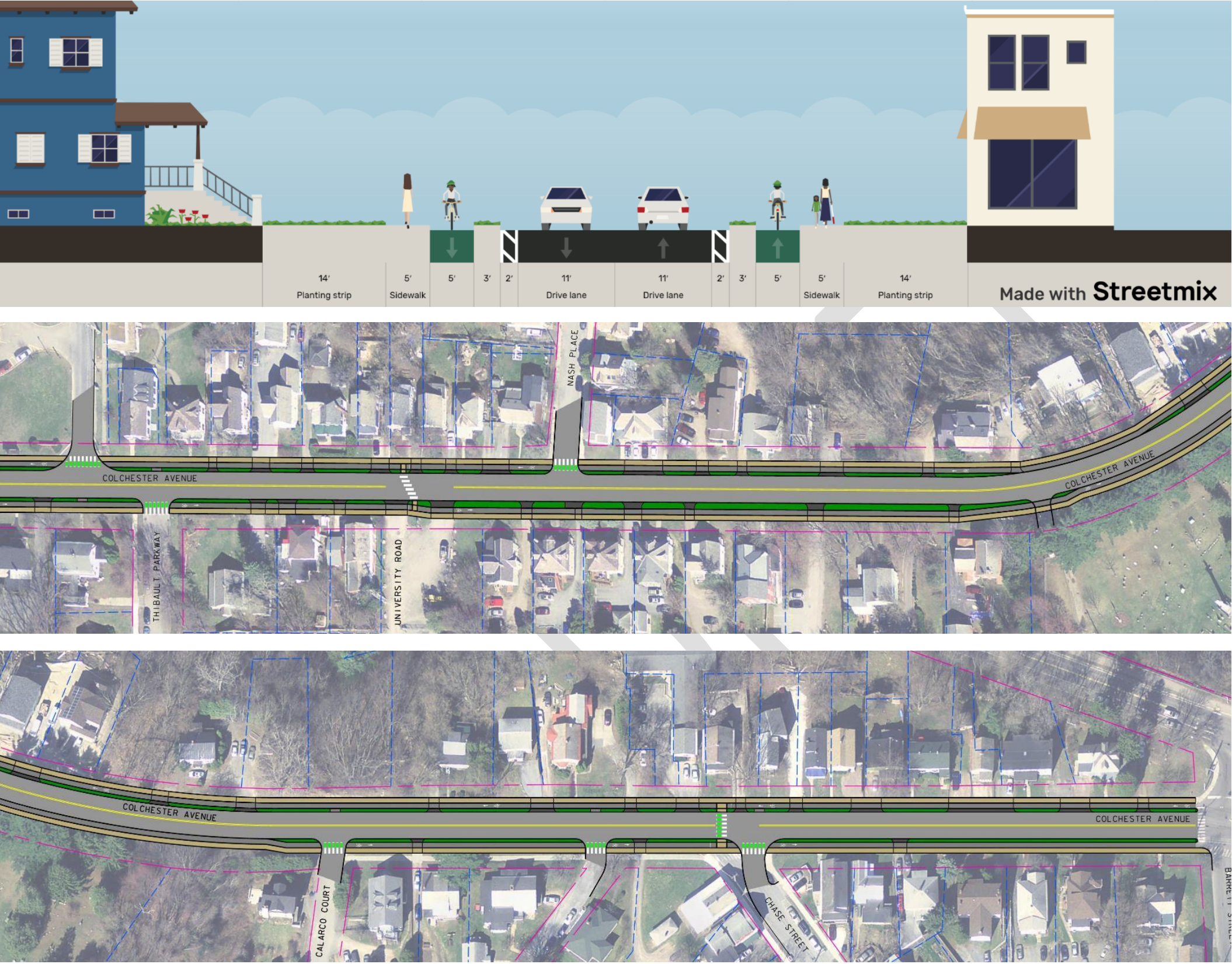
Figure 13: Colchester Ave Corridor Concept 2 (East): Raised, Separated Bike Lanes
