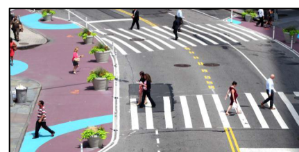
Figure 1: Examples of crosswalk improvements with paint, bollards, and planters
