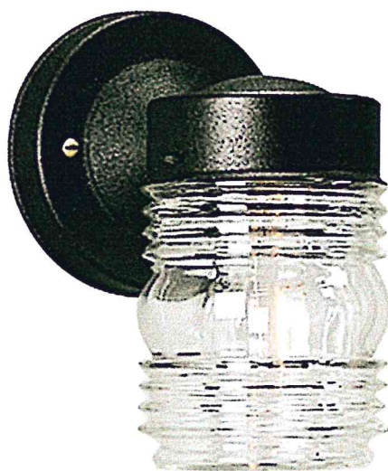
Photo 40. Light at apartment doors. Lamp will be an LED lamp with 2700K color temperature to match that of incandescent lighting. Width is 4.785" Height is 7.25". Housing is black.
