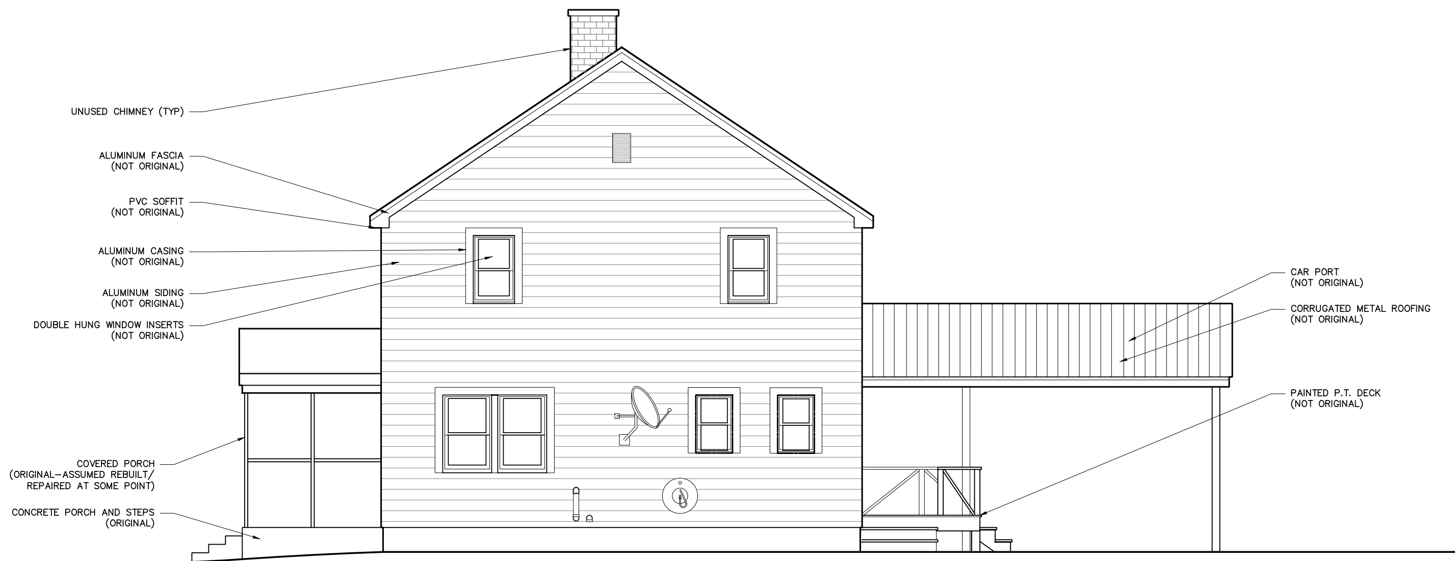
2 EXISTING WEST ELEVATION - SIDE
