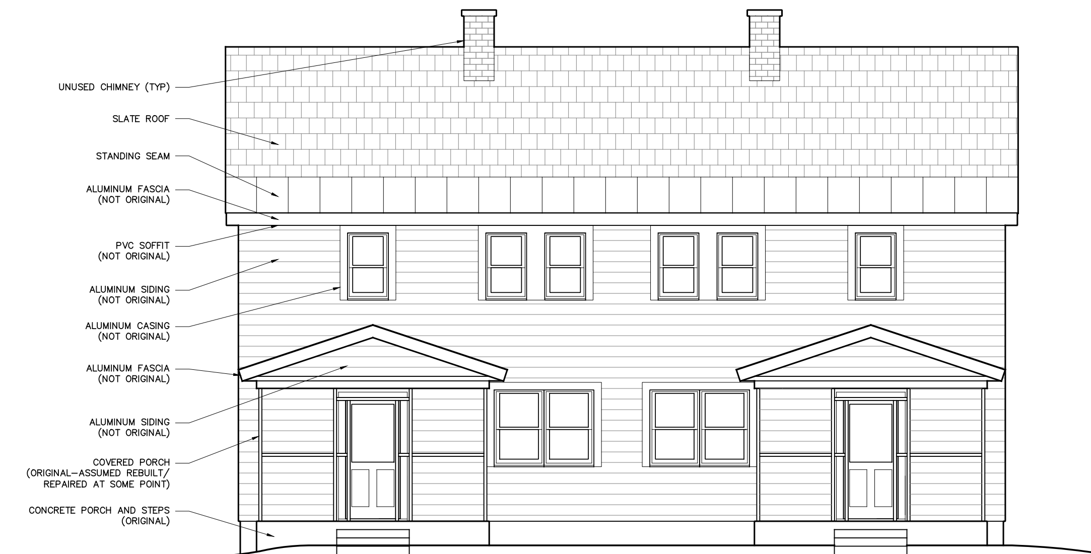
1 EXISTING NORTH ELEVATION - FRONT
