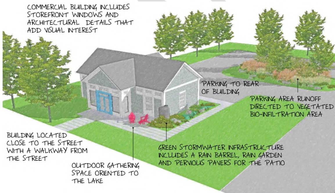
Figure 4-2. Building Placement and Design Standards Illustrated
