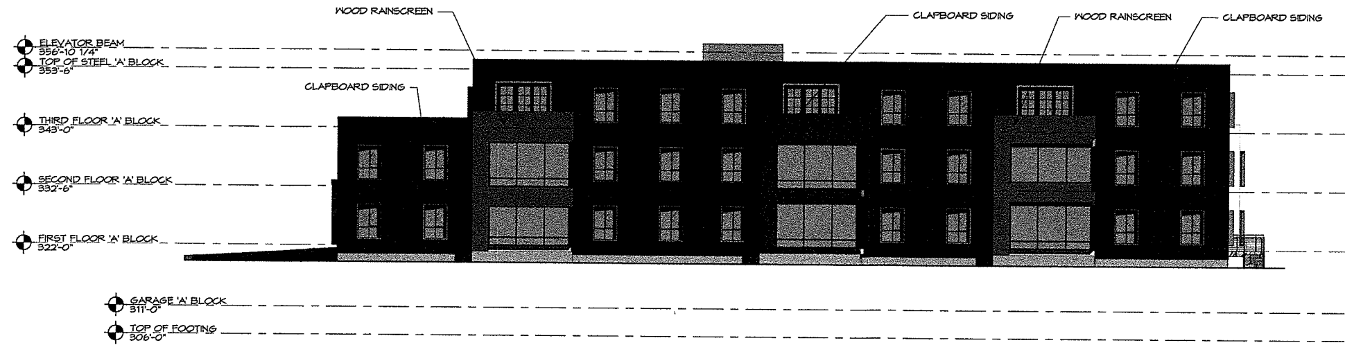
2 NORTH ELEVATION BLDG 2 3/32" = 1'-0" Referenced From A102
