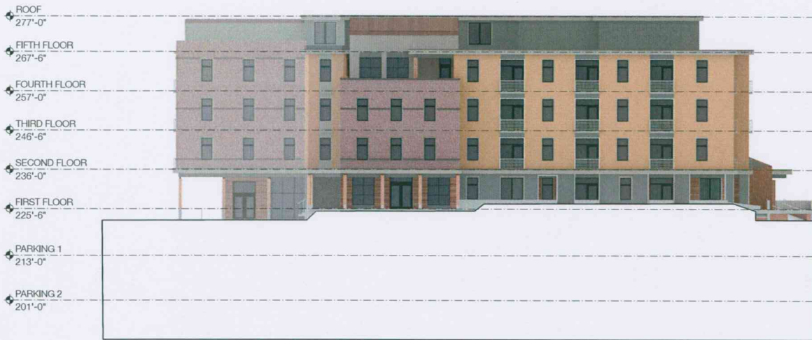
EAST ELEVATION Scale: 1/16" = 1'-0"
