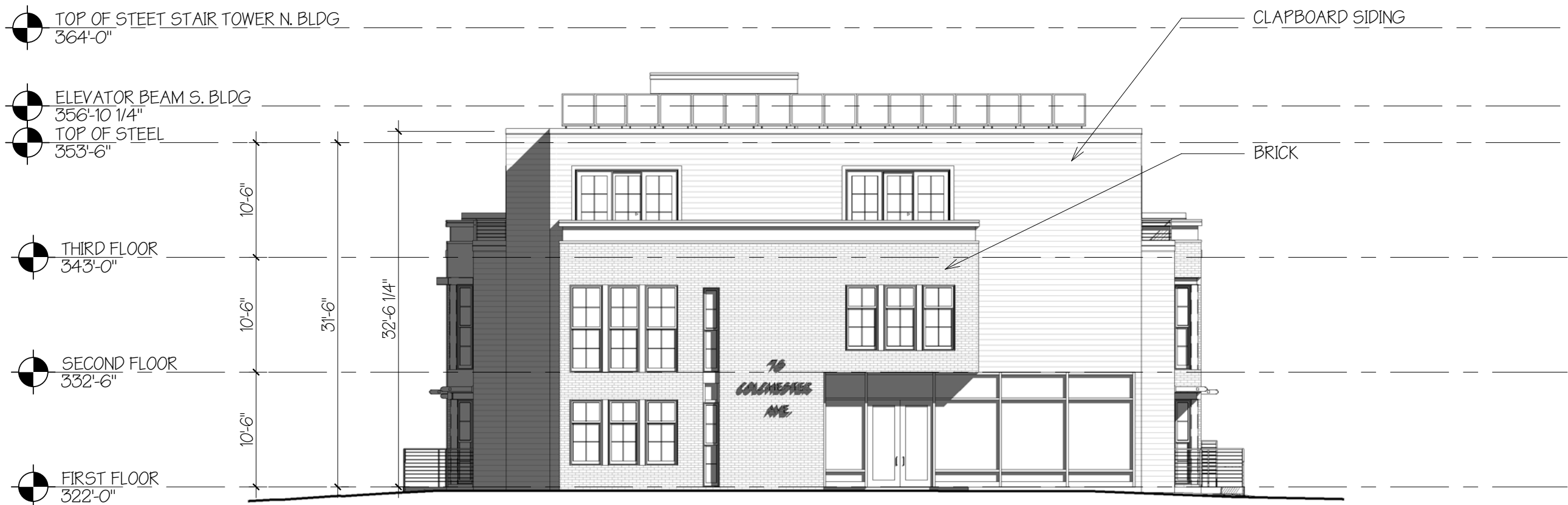
3 SOUTH ELEVATION BLDG 2 3/32" = 1'-0" Referenced From: A102
