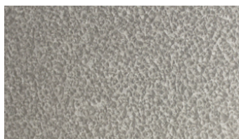
55% Al-Zn Alloy Coated Steel with Acrylic Coating (97)
