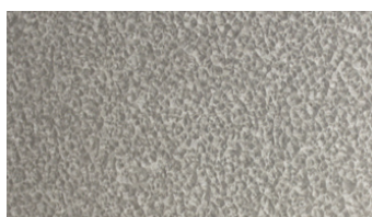
55% Al-Zn Alloy Coated Steel with Acrylic Coating (97)
