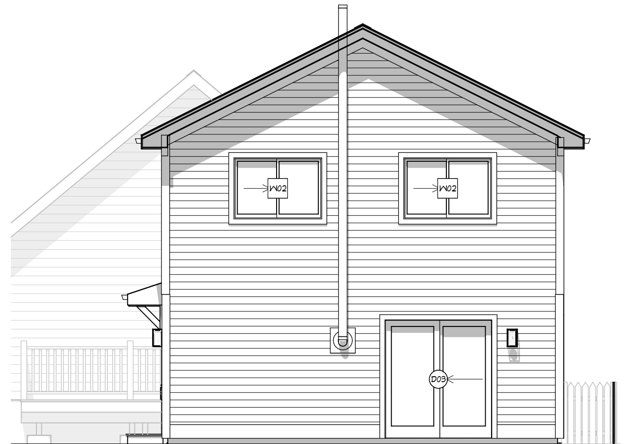
E4 WEST ELEVATION 3/16 in = 1 ft
