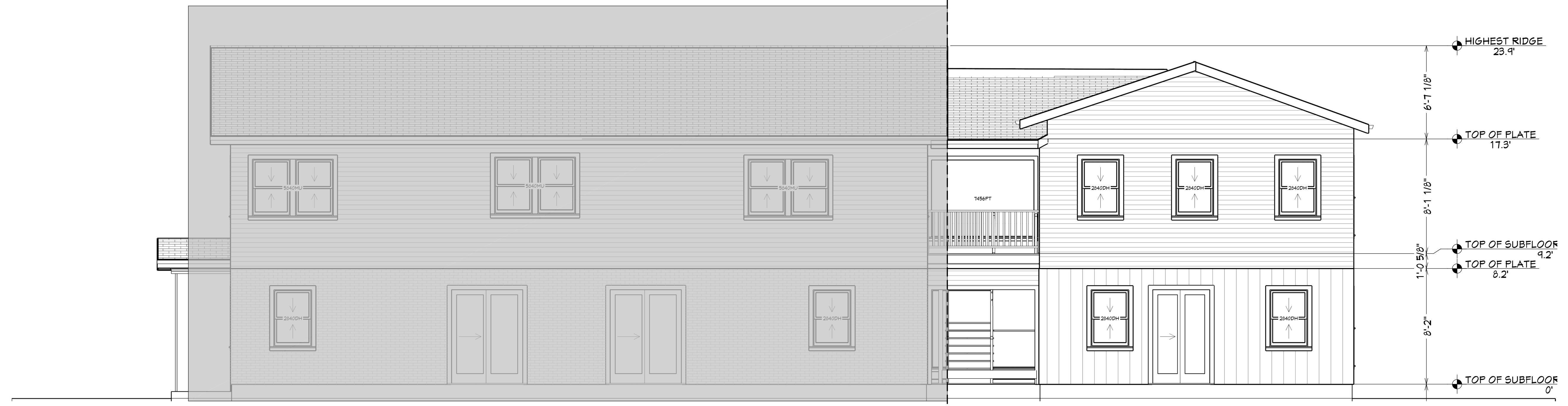
Exterior Elevation Back 1/4"=1'
