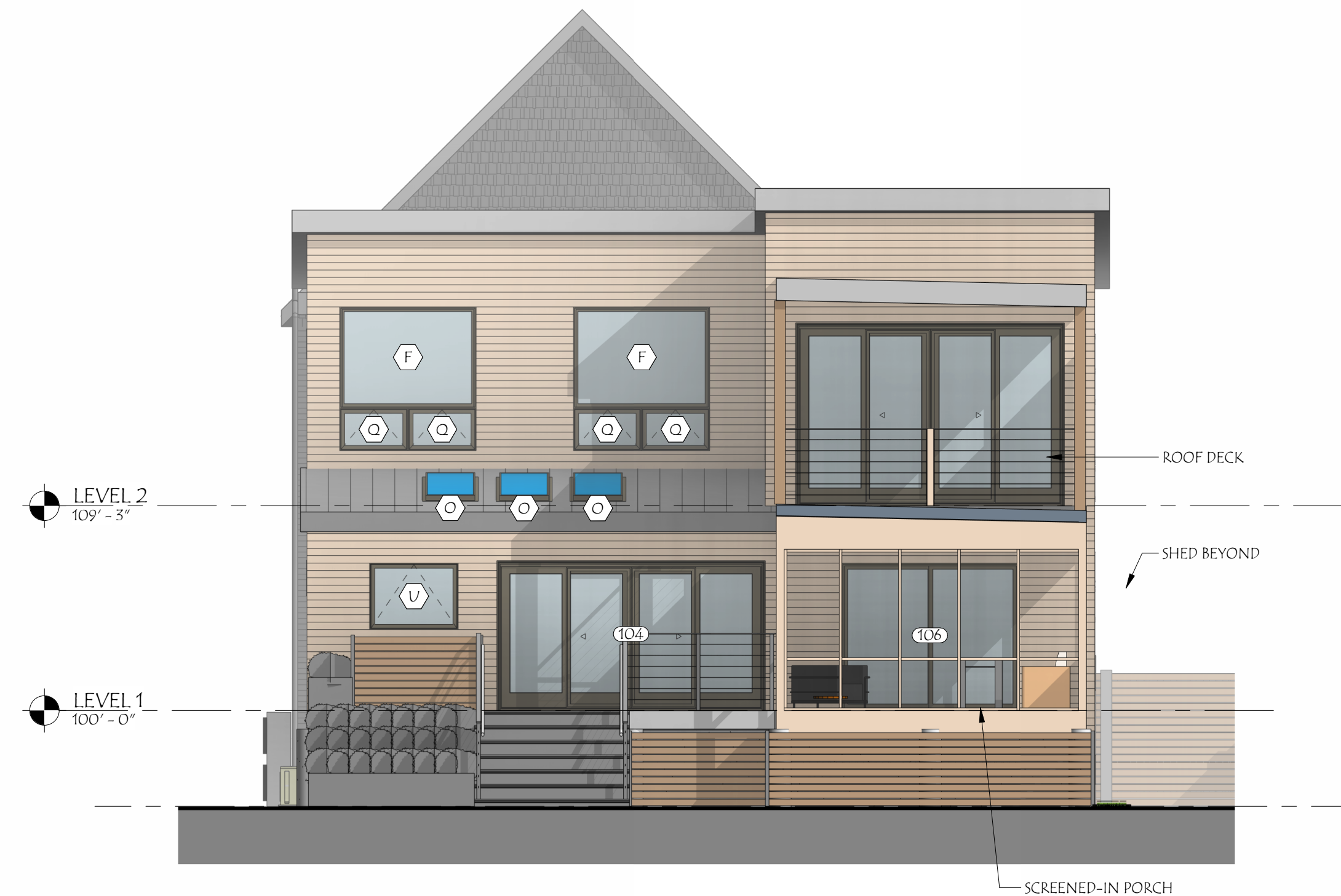
3 WEST ELEVATION SD-02 3/16" = 1'-0"
