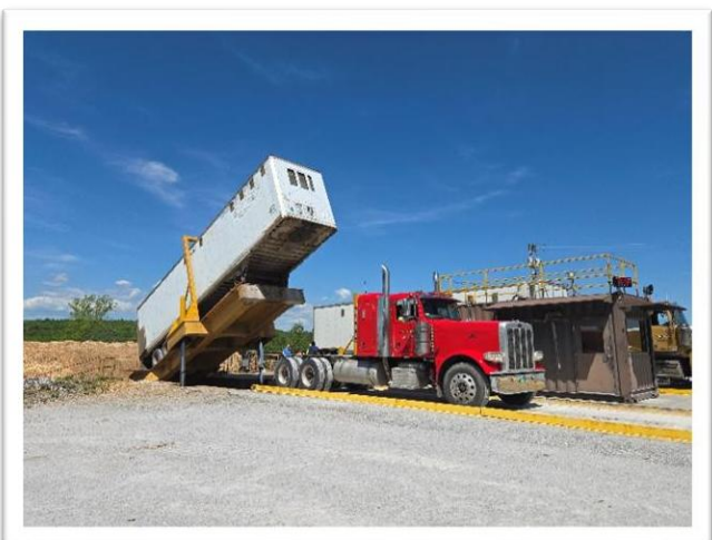
Photo 11: Swanton yard wood chip receiving station
