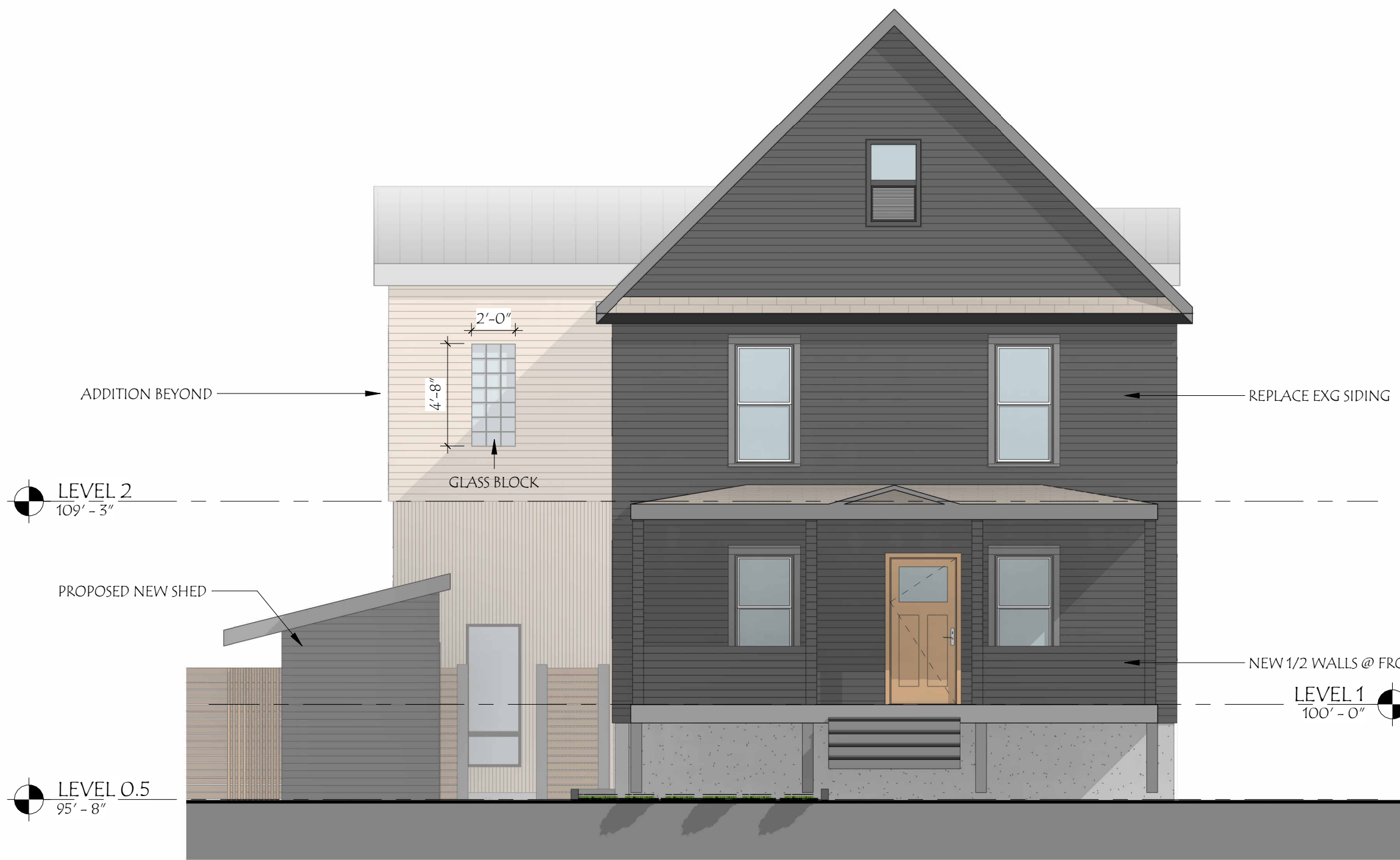
1 EAST ELEVATION SD-02 3/16" = 1'-0"
