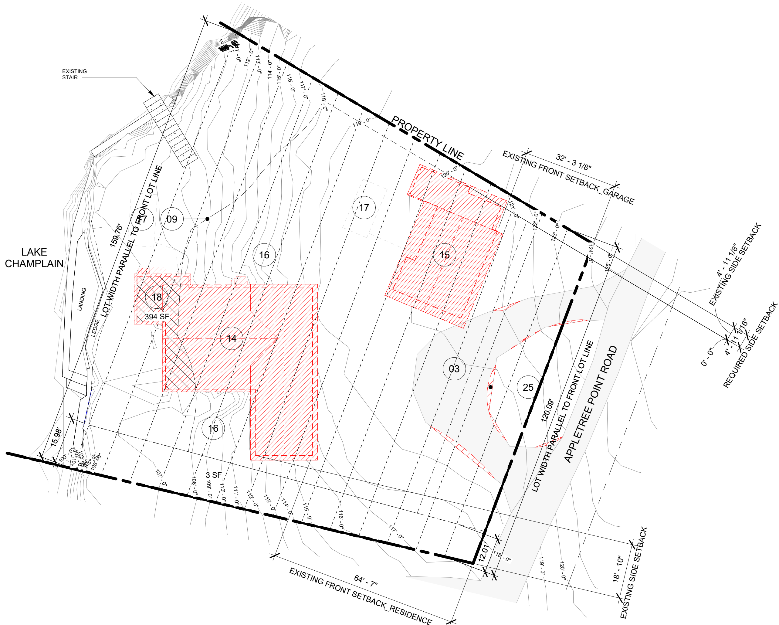
① SITE PLAN DEMOLITION ROOF PLAN 1" = 20'-0"
