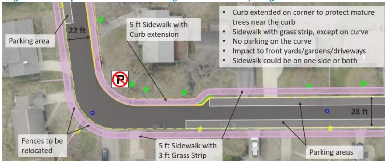
Figure 12 – Example of Alternative 3 Showing What a Preliminary Design on Both Sides of the Street
