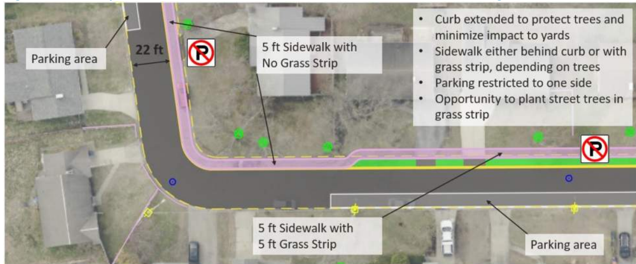
Figure 13 – Example of Alternative 4 with Sidewalk on Corner Outside of Existing Curb to Protect Trees
