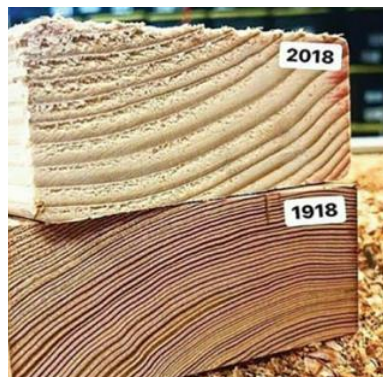
Figure 6. The dramatic difference in the number of growth rings between old-growth wood and wood that was recently harvested from second- or third-growth forests is indicative of the diminished dimensional stability and durability of most lumber currently available. Photo: Zachary Dettmore.
