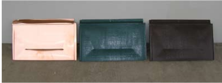
Figure 12—Copper and aluminum tiles—Zappone.
