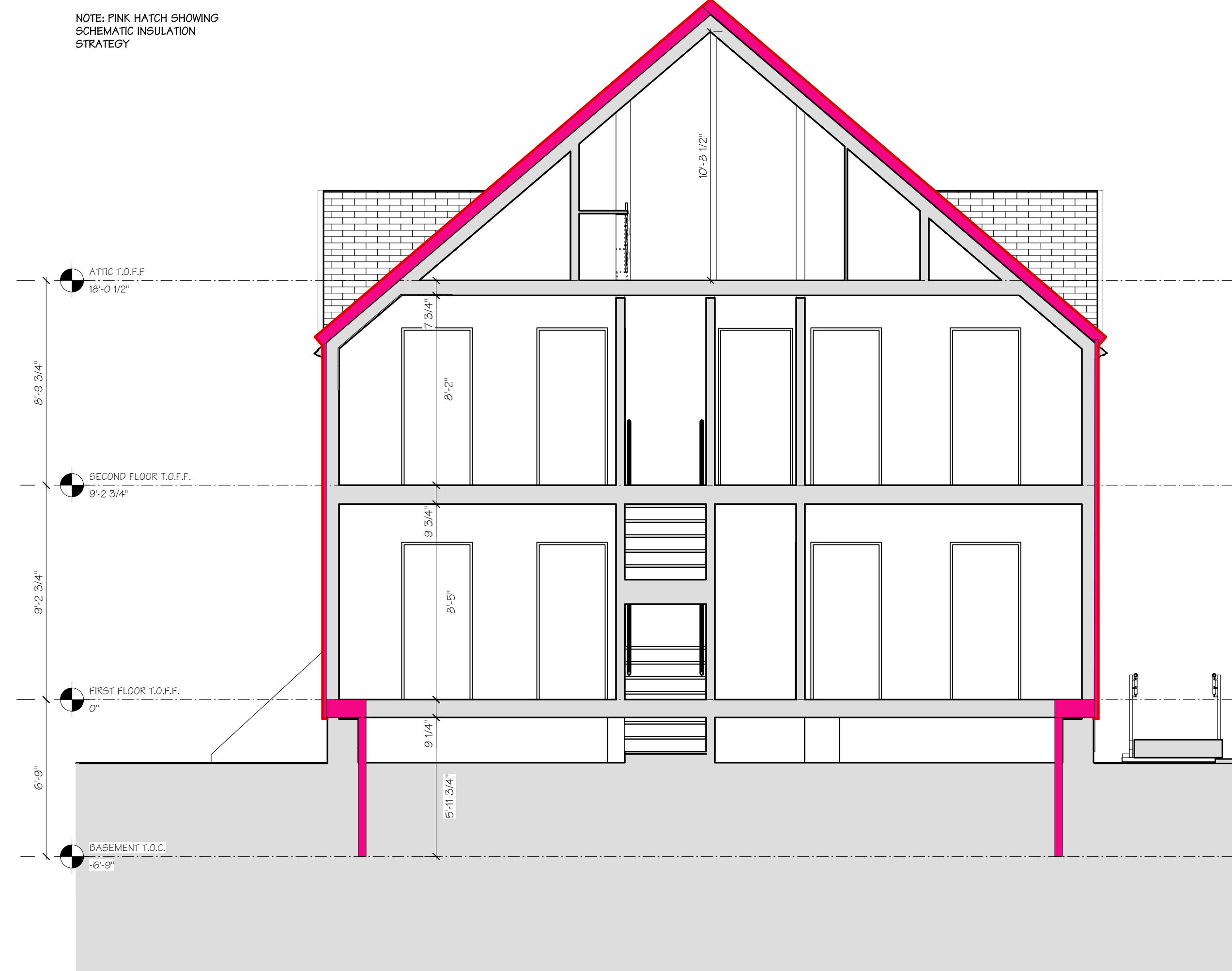
1 SECTION • EXISTING BUILDING Scale: 1/4" = 1'-0"
