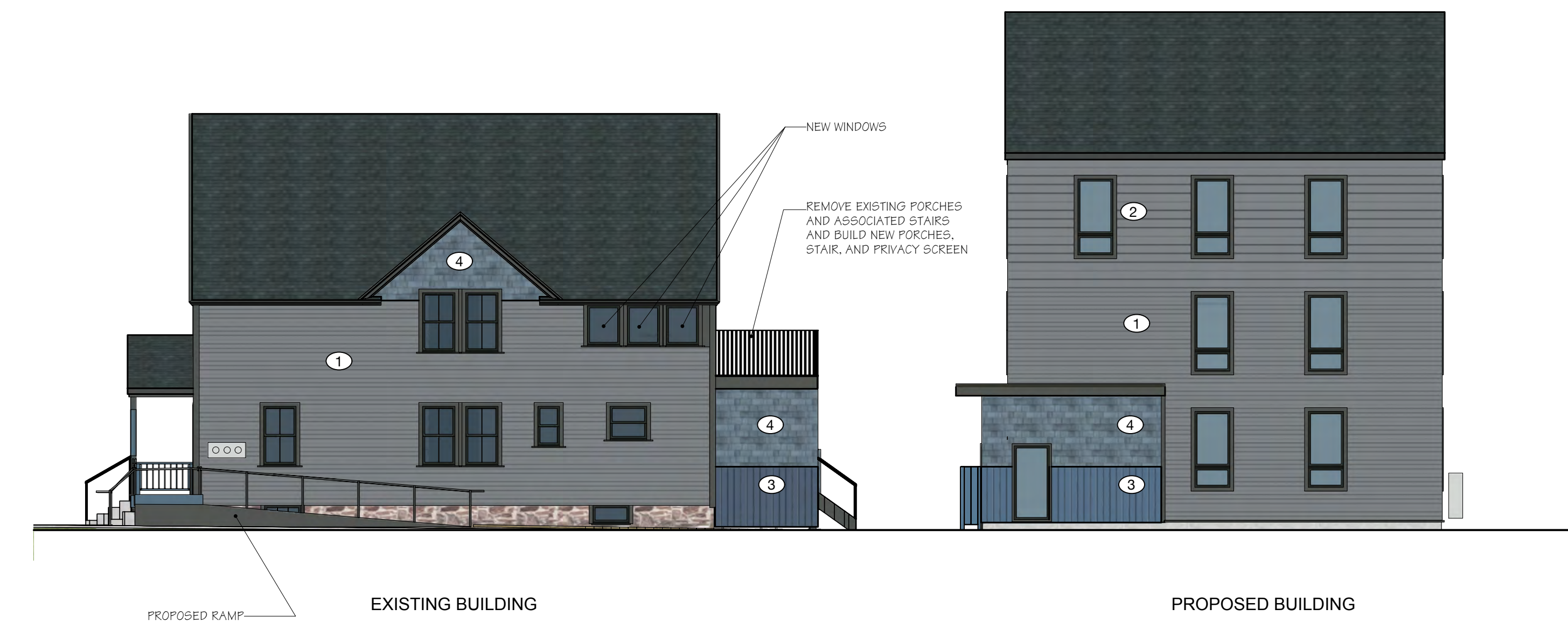
5 EAST ELEVATION • EXISTING AND PROPOSED BUILDINGS Scale: 1/8" = 1'-0"
